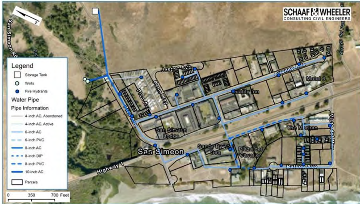
Figure 2. SSCSD Water System Overview
