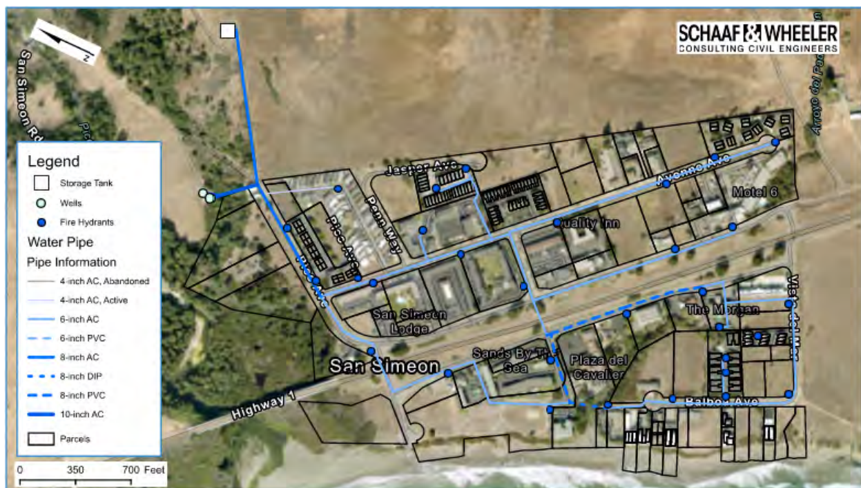
Figure 2 – Water System Overview
