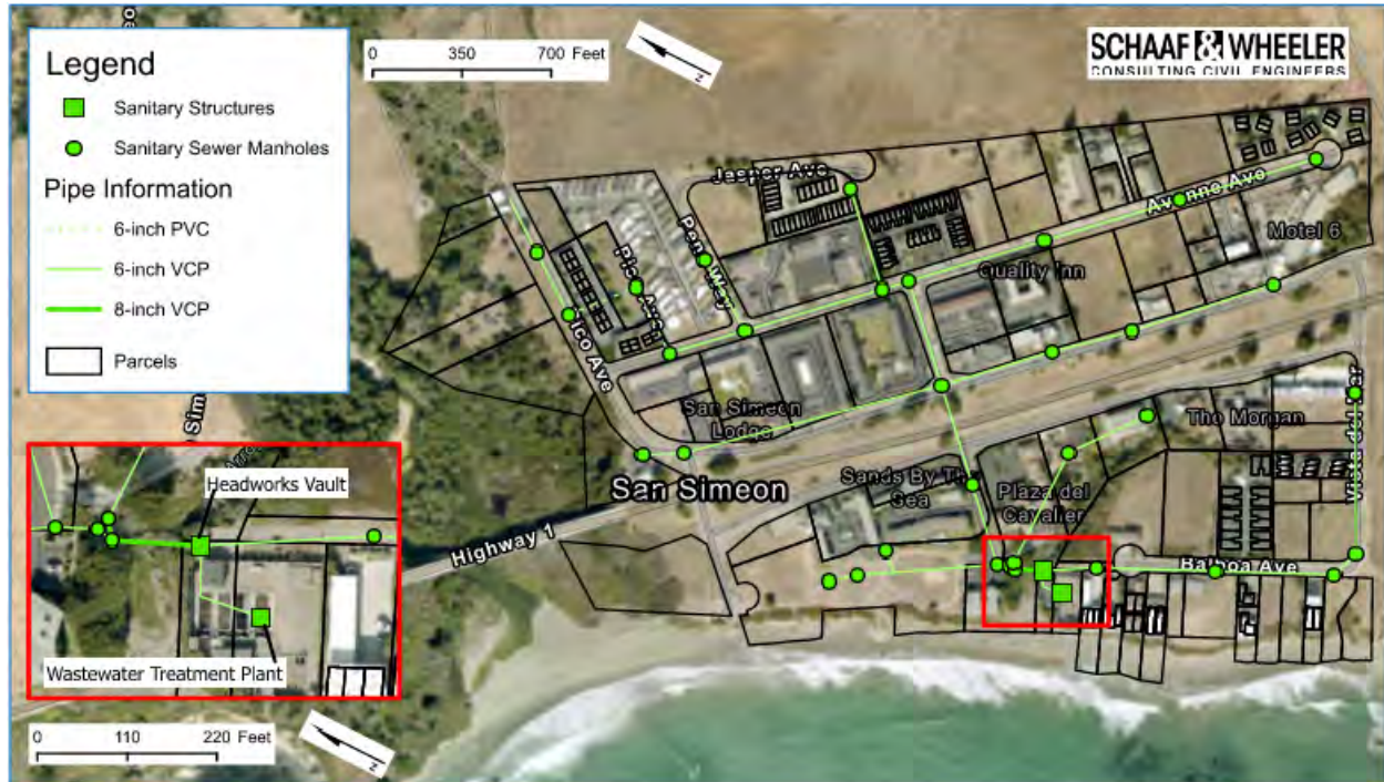
Figure 2 – Wastewater System Map
